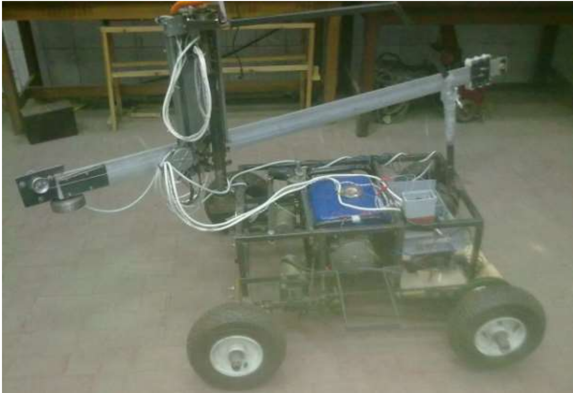
Figure 2.1: Robotic systems prototype designed to mimic human Deminer main movement
