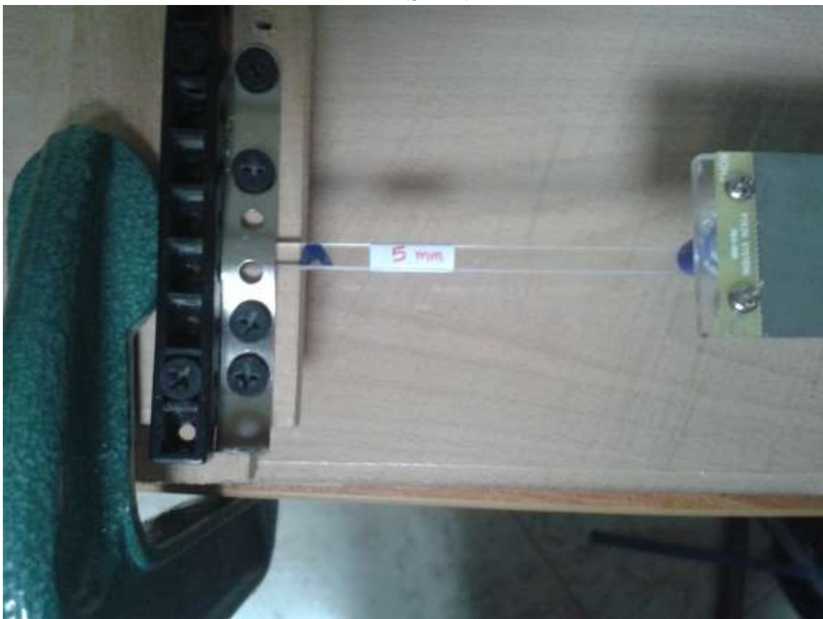
Figure 6.8: 5mm width specimen fixed in the final stiffness sensor setup
