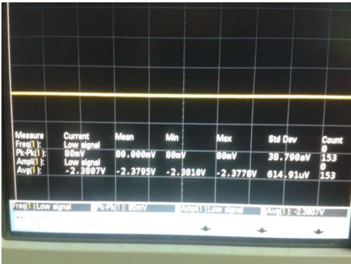
Figure 6.9: Oscilloscope output no excitation exist, noise only exist.
