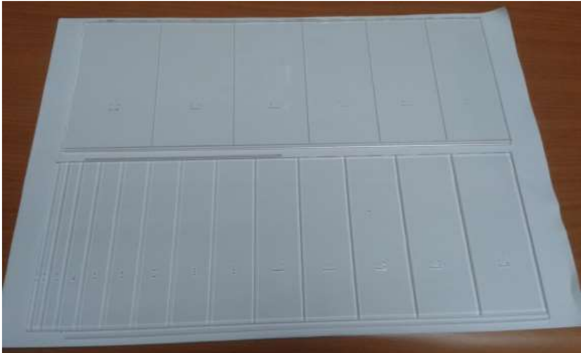
Figure 6.7: Twenty specimens fabricated with widths from 2.5 mm to 22.5 mm, with step 2.5 mm.
