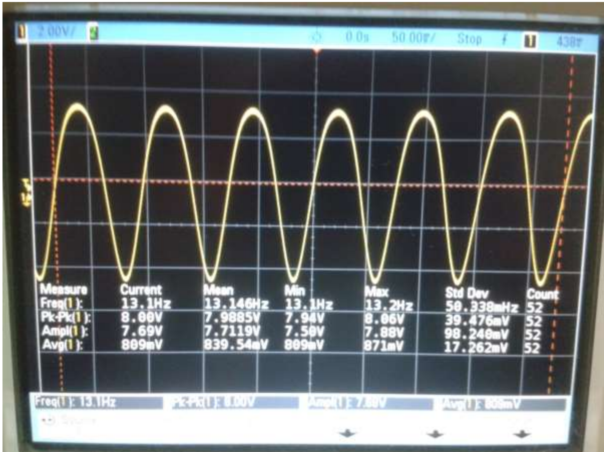
Figure 6.10: Oscilloscope output at k_o=0 , and with excitation at 1 st resonance mode.
